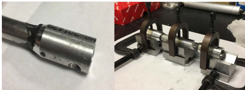
Figure 2. 1 a (left): Sample adapter nut adhered to the end of sample tube. b (right): Supportive V-block setup to allow adapter nut curing.
