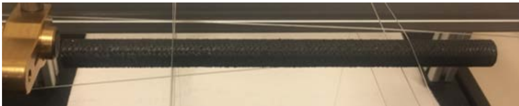
Figure 2.11: Recording setup for longitudinal vibration via table mounted IE
