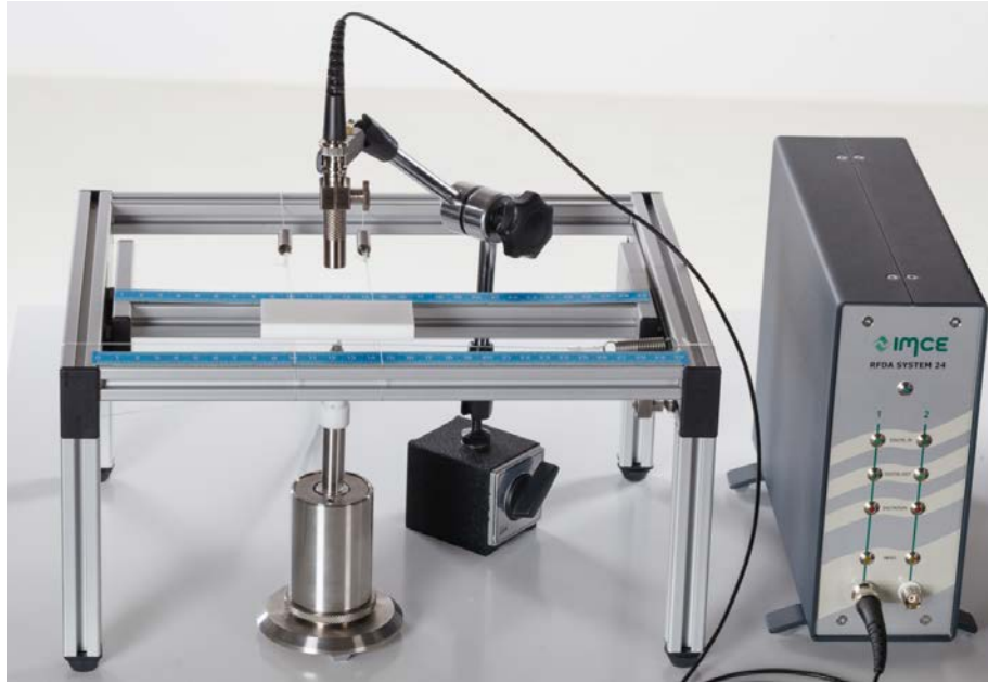
Figure 2. 9: RFDA System 24 hardware used for IE testing [64]
