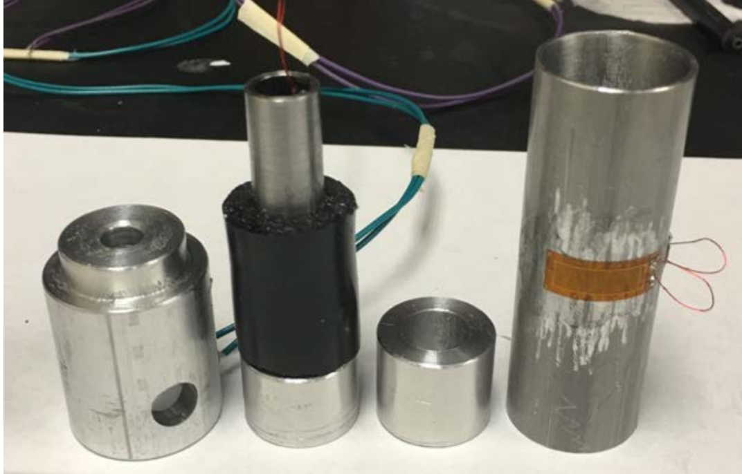
Figure 2. 19: Image of parts required for expanding plug test for external pressure
