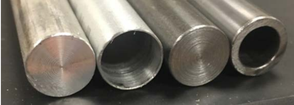
Figure 3.4: Materials used to validate rig mounted impulse excitation. (Left to right) Al 6061 Rod, Al 3003 Tube, 4140 Steel Rod, and 4140 Steel Tube.
